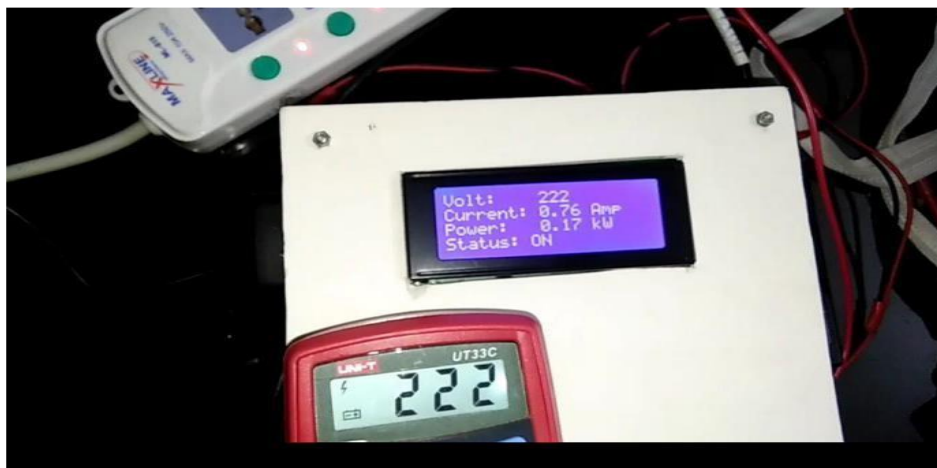
Figure 5. Status “ON”, Volt: 222 V, Current: 0.76Amp, Power: 0.17 KW
